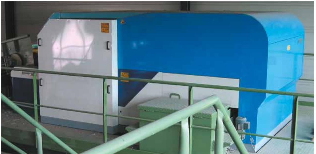
After being well separated into single pieces, the paper is conveyed to the recognition and illumination unit and thus passes the sensors. In this area the flow of materials is taken over by the optical recognition system and at the same time analysed by the computer, which determines the colour and degree of print.
