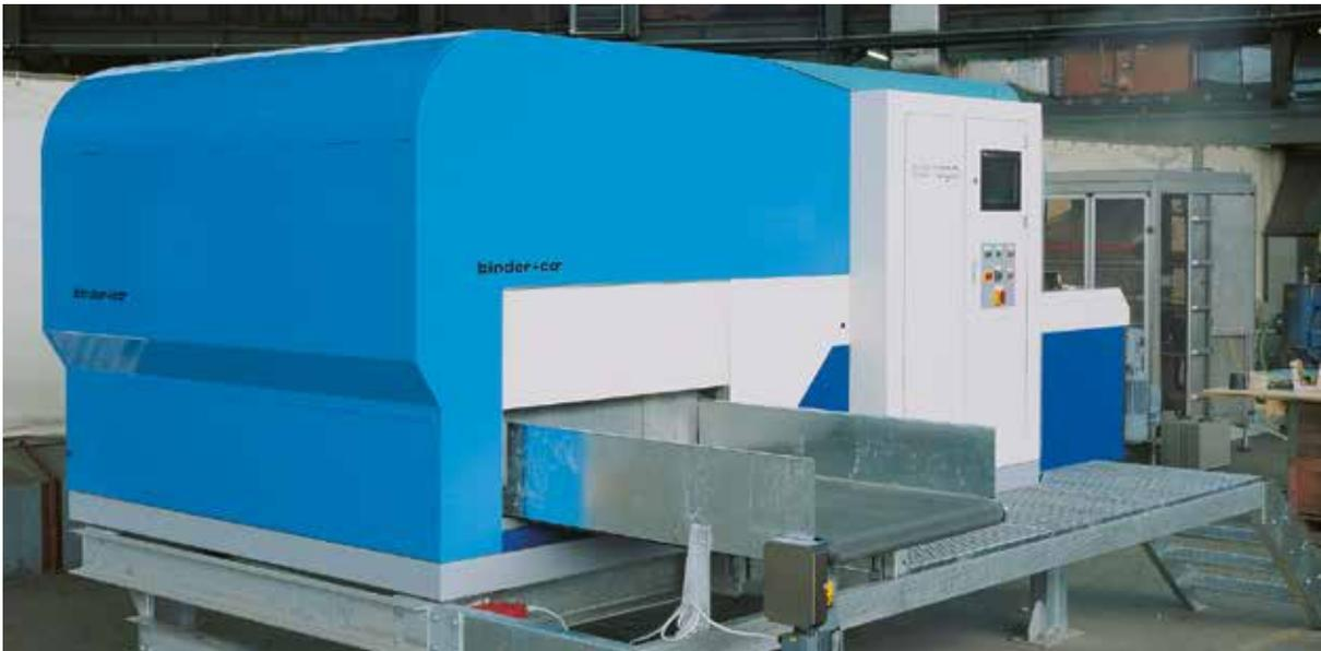
CLARITY is used primarily for sorting cardboard from waste paper materials in industrial and communal collection systems. A prerequisite for optimum operation is an even-as-possible size of pieces to be sorted and a one-layered charging evenly distributed over the width of the machine. This is achieved by pre-sorting and using a special feeder system.
